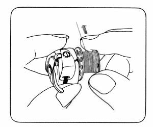
Guide thread into slot (a) of bobbin case.
